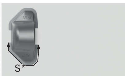
Pic. 1: Weld on welding block 1
