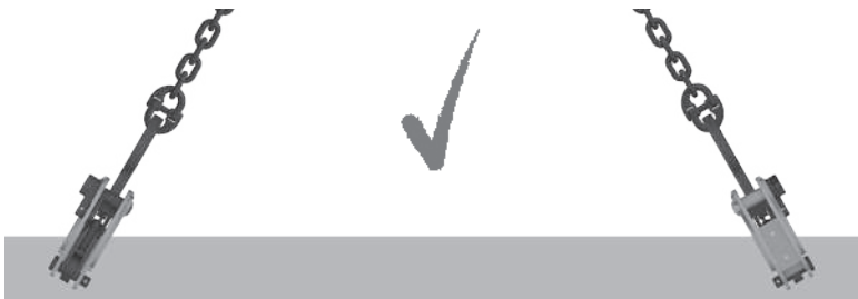
Fig. 6: Permitted load: Clamp in line with cord
