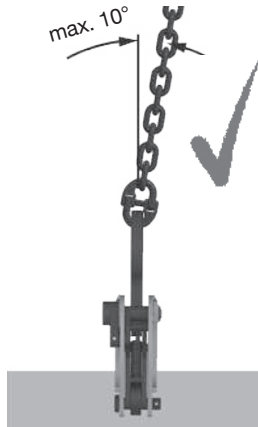
Fig. 4: Maximum permitted Transverse load: 10°
