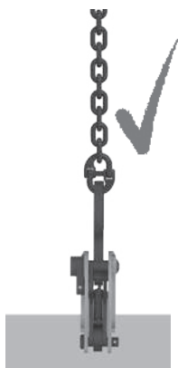
Fig. 11: Charge horizontale optimale max. 10°
