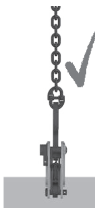
Fig. 11: Optimum horizontal load
