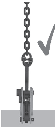
Fig. 3: Optimum horizontal load
