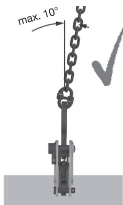
Fig. 12: Maximum permitted Transverse load: 10°
