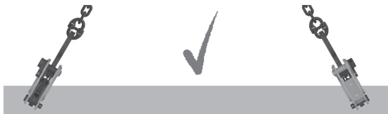
Fig. 14: Permitted load: Clamp in line with cord
