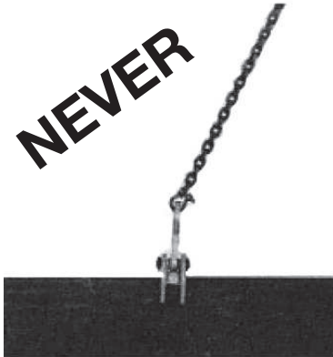
Photograph D (Typical) Excessive side loading.
